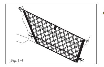
(e) Confirm completed assembly. Make sure net handle is facing out toward the rear of the vehicle (Fig. 1-4).
